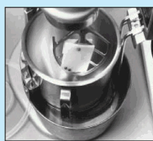
2. Placement of high-density polyethylene coupon on space-shaped agitator blade
