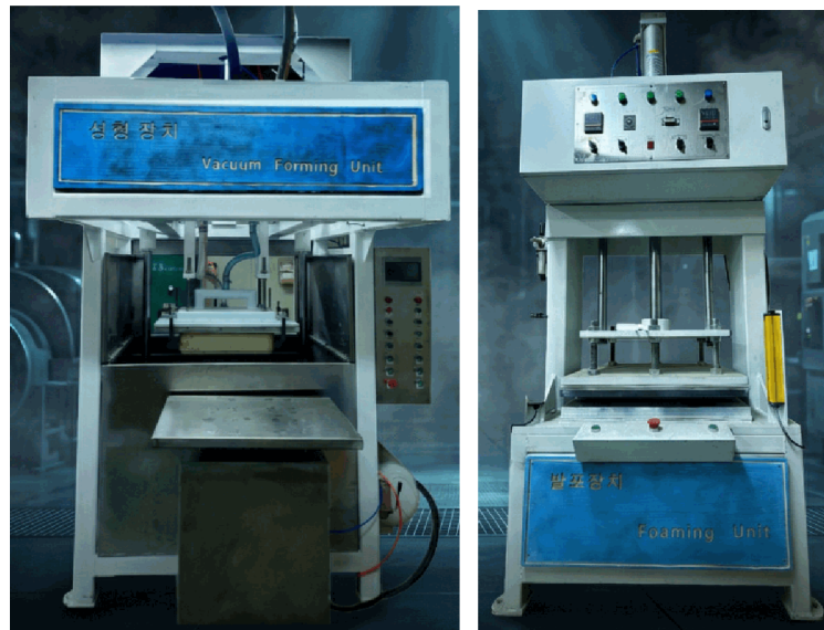
Fig. 2. Pilot-scale cellufoam manufacturing system: left: vacuum-forming unit; right: foaming unit. core processing equipment for the high-temperature and high-pressure cellulose foaming process utilizing pure natural pulp.
